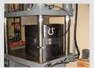
First, high capacity load cells are often integrated into a machine, system, or structure with little space in which to install the sensor. As a result, heavy duty load cells should be designed to be compact, small, and light in relation to their capacity. We have designed and built high capacity load cells as small as six inches in width and one inch in height.
