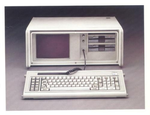
And software can always be close at hand: The system's front panel contains a compartment for storing program and data diskettes.
