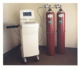
Praxair argon and helium for Endocare's Cryocare System are nontoxic, nonflammable, and inert. Material Safety Data Sheets (MSDSs) are available on www.praxair.com/msds listing gas, hazards, characteristics, and valve connection data.
