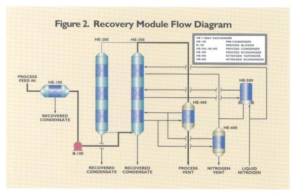
In the KRYOCLEAN recovery module, dual process condensers cooled by liquid nitrogen are used to condense volatile organic compounds so they can be removed as liquids.
