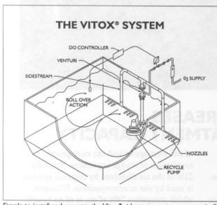
Simple to install and operate, the Vitox® sidestream system automatically controls dissolved oxygen in activated sludge basins.
