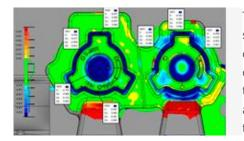
Trinity Forge is a closed-die forging plant that specializes in complex shapes in a wide variety of sizes. To meet the stringent specifications of their customers, Trinity uses the FARO ScanArm daily to inspect dies when they come off the CNC machines, to track die wear, and to reverse engineer products that may not have prints or legacy data available. The speed at which they can now operate is a great value to the company.
