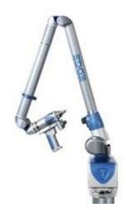
The FARO ScanArm is a portable CMM ideally suited for reverse engineering applications. Non-contact measurement is usually a faster way to inspect and measure parts, and industry as a whole is moving away from hard probing toward laser scanning. One key advantage of laser scanning is that soft, deformable, and complex shapes can be easily inspected without coming into contact with the part.
