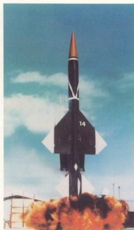
Below: Boeing's BOMARC missile system utilized the world's first operational pulse doppler airborne radar, which was designed and produced by Westinghouse.
