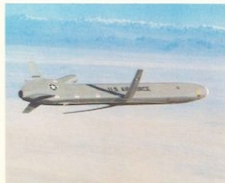
Below: Litton's LN-35 inertial navigation element guides and controls this Boeing cruise missile.
