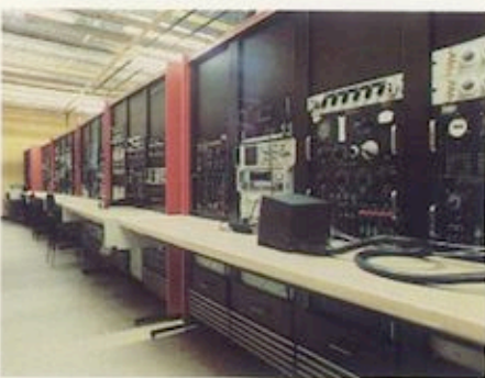
Above: Air defense systems are demonstrated and integrated at the Westinghouse command and control simulation laboratory before being shipped to the customer.
