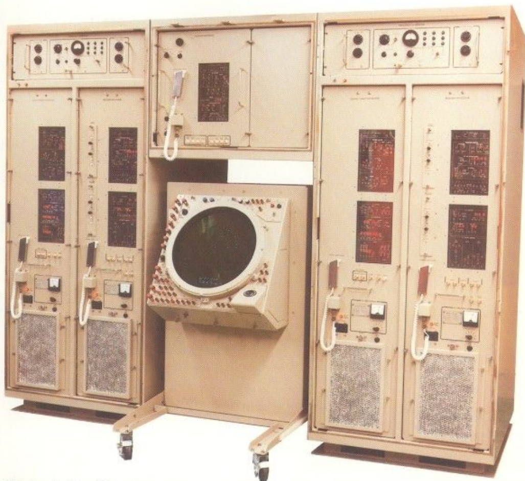
The two inside cabinet drawers contain dual receiver/processors which can provide simultaneous display of several different video modes.
