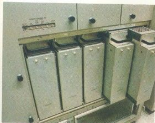
Full power can be maintained even if one of these five independent switches in the ASR-30's solid-state modulator should fail.
