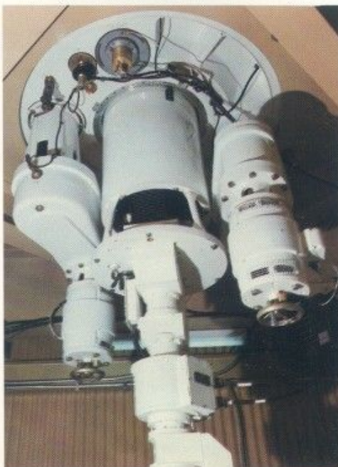
An offset beacon feed is placed to the side of the radar horn to provide the desired beacon pattern without degrading radar performance.
