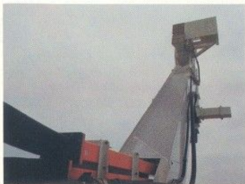
An offset beacon feed is placed to the side of the radar horn to provide the desired beacon pattern without degrading radar performance.
