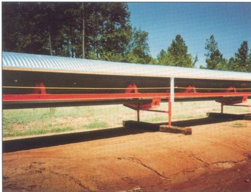
Belt capacity is 1,500 tons per hour at 800 feet per minute. Belt width is 36 inches.
