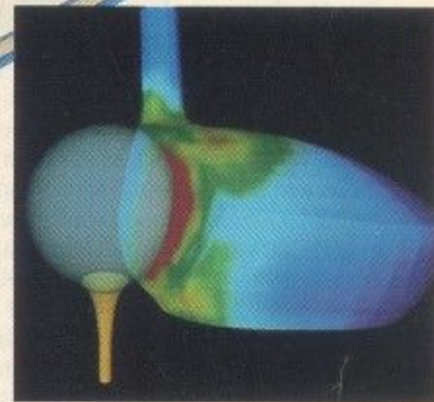
A view of a golf club hitting a ball shows the distribution of stress at the moment of impact.
