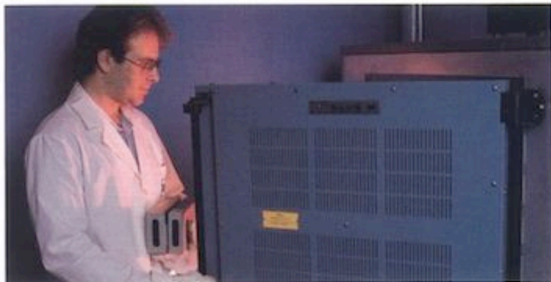
Here, a Conductimer adhesive is subjected to temperatures of 150°C for 2,000 continuous hours to test performance under accelerated aging conditions.
