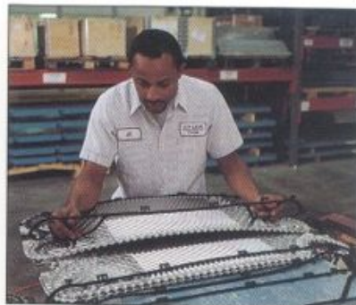
Clip-on, glue free gaskets are applied
