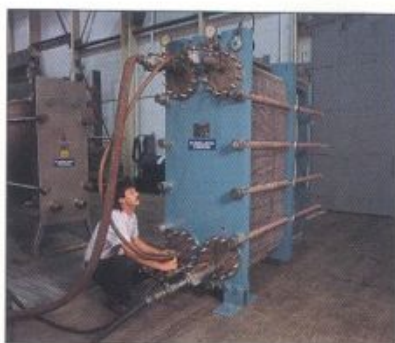
Hydrotest. Using pressurized water at one and a half the design limits, finished units are tested before shipment
