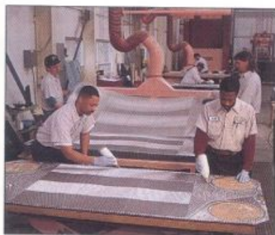
Gluing procedures include oven curing for maximum bonding
