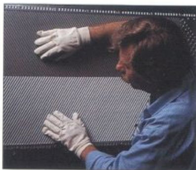
Light box inspects plates for imperfections
