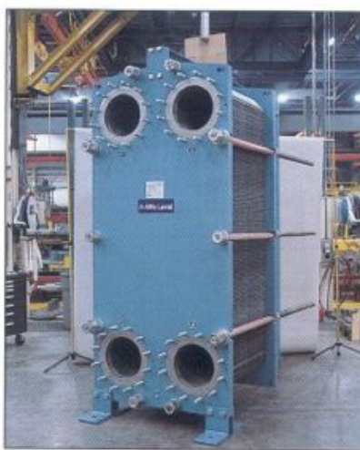
Thicker frame covers and fewer tightening bolts are characteristic of today's Alfa Laval plate heat exchanger.
