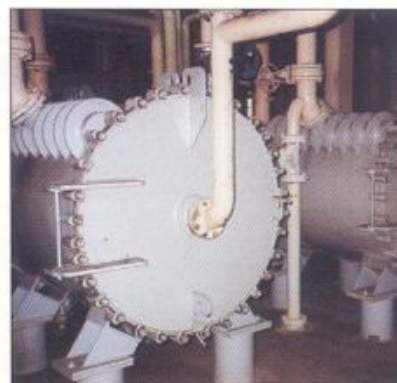
For two-phase, slurries and other difficult applications, Alfa Laval spiral heat exchangers are an effective alternative.
