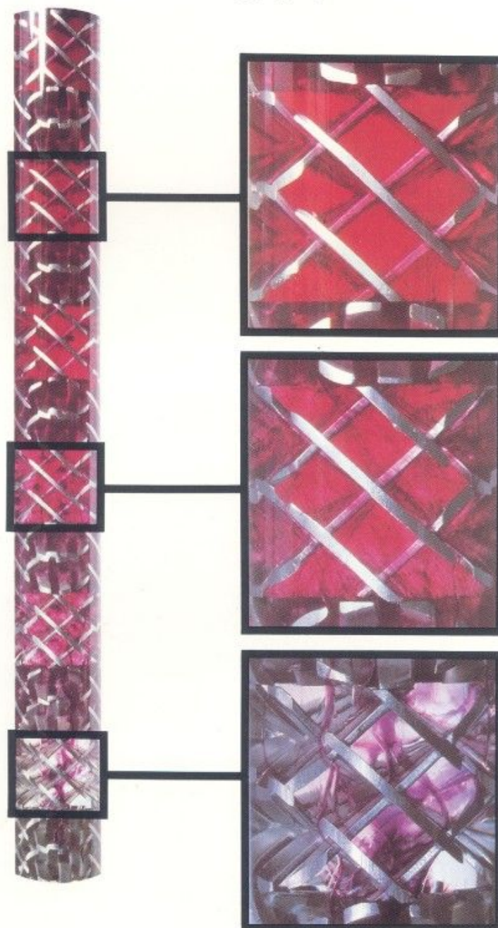
FIG. 11 Mixing water (dyed red) with glucose is accomplished in a relatively short mixer length.
