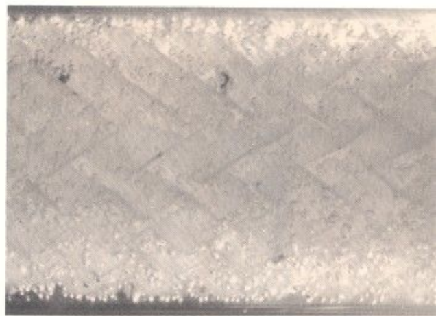
FIG.24 SMV elements generate a bubble bed in air-water contacting.
