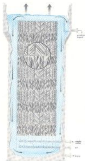
FIG.25 In the Koch gas-liquid reactor, static mixing packing breaks the gas into fine bubbles and disperses them uniformly throughout the liquid.
