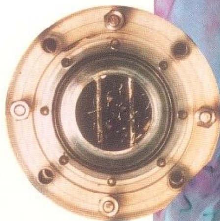
FIG.5 Typical retainer assembly (above) for a Koch static mixing unit.
