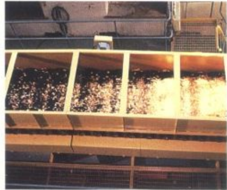
A key requirement of chip screening is to prevent loss of usable fiber. RETEC chip screening systems are designed to meet this requirement with special "flip-flow" screens that recover pins from the fines chip flow and return the pins to the accept material flow for pulping.
