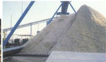
RETEC was one of the first companies to offer traveling screw reclaimers to the North American pulp and paper industry, and today RETEC's TSR™ is the most widely used traveling screw reclamation system. A tapered screw pulls chips evenly from the various layers in the chip pile, ensuring uniform in-pile blending.
