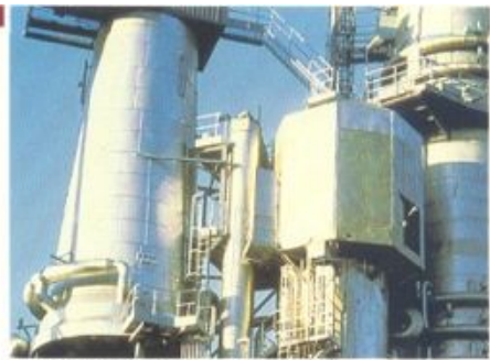
RETEC's presteaming system increases digester capacity, allowing higher quality pulp to be made using less energy.
