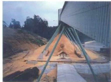
In Chile, RETEC designed an open-air storage system for hardwood and softwood using two TSR-16 reclaimers and an overhead stack-out conveyor.
