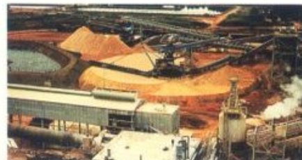
RETEC's V-V Stacker/Reclaimer is built specifically for the "continuous-use" requirements of the pulp and paper industry. An oversized center bearing simplifies maintenance and enhances system reliability.
