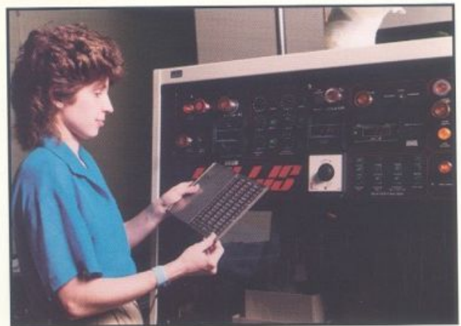
Waveless solder machine applying solder finish to leads on high-rel parts. The machine slowly passes the leads through a hot solder bath to ensure that a uniform layer of solder is applied.
