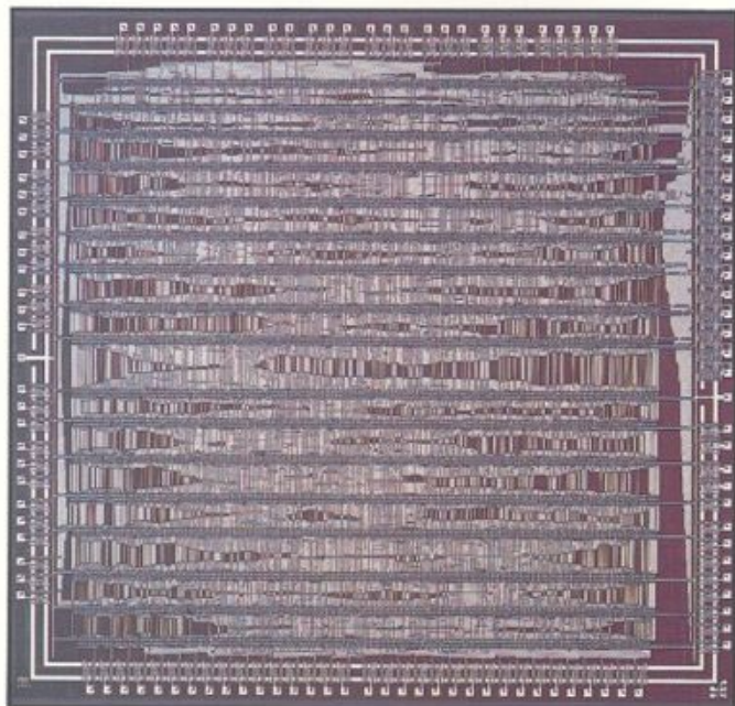
Photo of an ASIC made with radiation-hardened CMOS/SOS standard cells.
