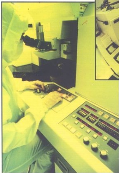
Projection aligner uses a series of intricate mirrors to automatically align and expose wafers.
