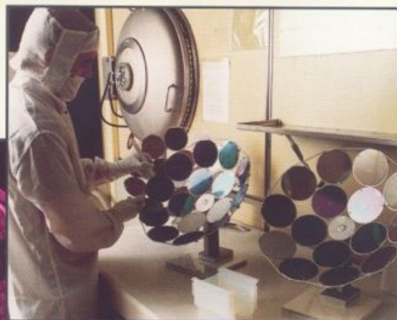
Wafers are loaded on planets to expose surface to an atmosphere of evaporated aluminum. Wafers are coated to a specific thickness that later will be exposed to an etch pattern that leaves thin lines of aluminum metallization.
