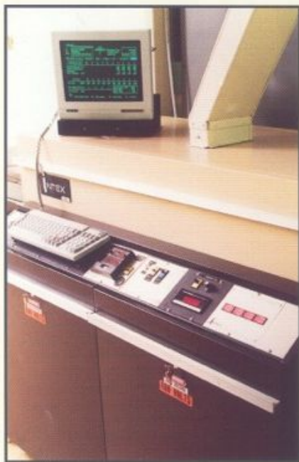
Frame sink furnace seals units in a clean-room atmosphere using infrared rays to heat the epoxy and quickly seal the cover to the frame.
