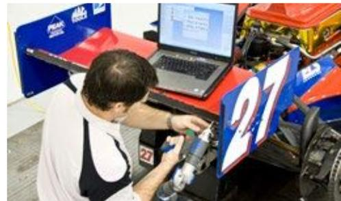
Having FARO in-house enables Andretti technicians to measure and inspect parts, scan models, and verify set-ups. It also eliminates the time and expense of paying outside service providers to do their reverse engineering measurements.
