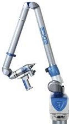
The FARO ScanArm is a portable CMM ideally suited for reverse engineering applications. Non-contact measurement is usually a faster way to inspect and measure parts, and industry as a whole is moving away from hard probing toward laser scanning. One key advantage of laser scanning is that soft, deformable, and complex shapes can be easily inspected without coming into contact with the part.
